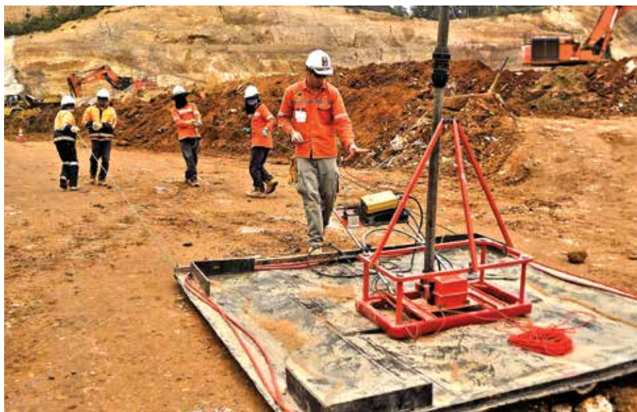
Laneville directs his team in dragging his mine-detecting device (Modified EM61 with 2-turn transmitter) near mineral exploration sites around Sepon, Laos, home of the country’s largest gold and copper mine.
